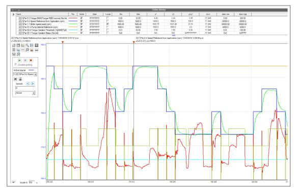
86.03 Cavitation Fault/Alarm is set to Alarm and 86.10 End of Tank Detection to Enabled.
