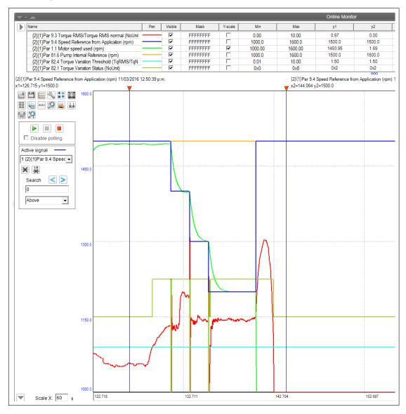
• The drive detects cavitation occasionally and the speed goes up and down. At minimum speed, the program detects cavitation for a time that is shorter than 86.07, so the drive does not trip.
